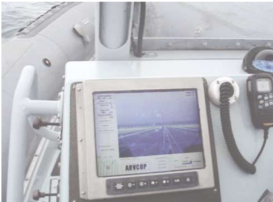
Figure 5: Real Time Track Overlays Provide Unique Conning Guidance to the Craft Operator
