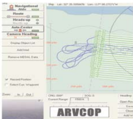
Figure 4: Recorded Track of 11m RHIB (10m spacing) in Cross Current, Low Visibility Conditions. The screen shows the Gods Eye View in the main display with the AR image in the lower portion. These Displays can be swapped between both screens.
