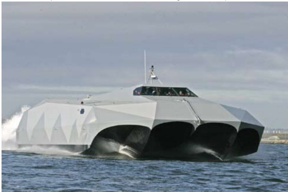
Figure 1: Stiletto, an Experimental USN Hull Form used in Howler
